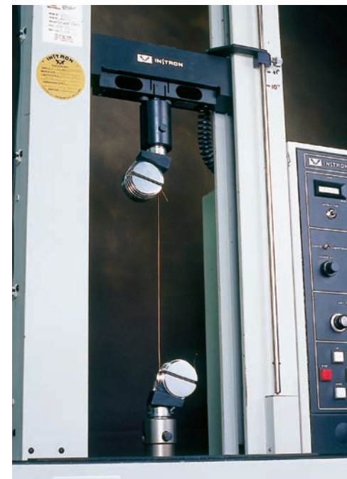
Quality control inspections include testing incoming wire shipments for tensile strength and elongation.
